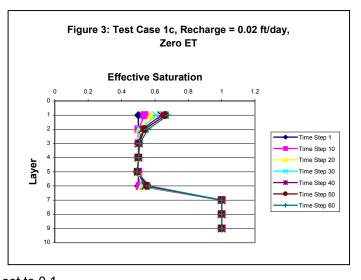
These illustrative cases were run as transient simulations with one 30-day stress period broken up into 60 equal time steps. The grid was subjected to constant recharge in the top layer and no evapotranspiration. In test cases 1a, 1b, and 1c, recharge was set to 0.3 ft/day, 0.04 ft/day, and 0.02 ft/day, respectively.
