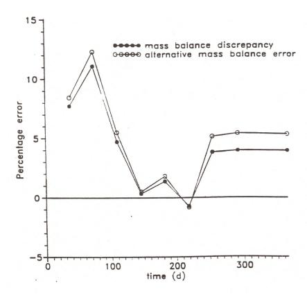
Figure 2. Mass balance errors versus time
